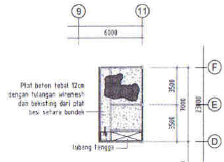
DENAH PLAT BETON LANTAI 2 SKALA 1:250
