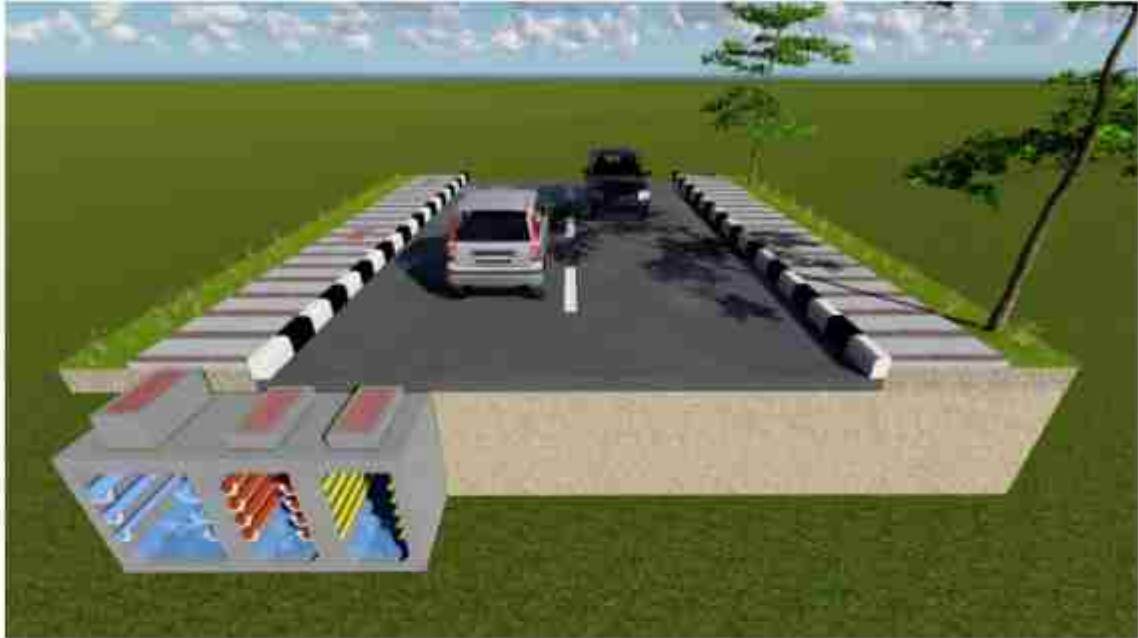
Gambar 5.42 Perspektif ducting tanpa drainase
