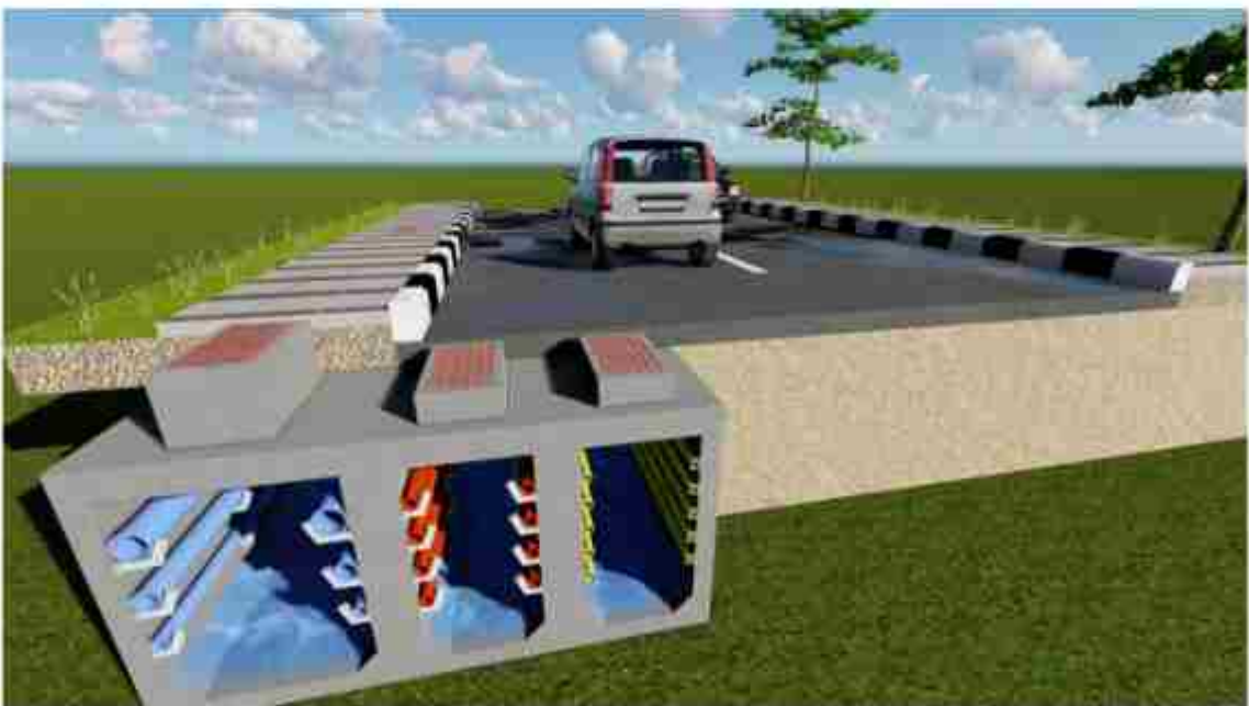
Gambar 5.43 Perspektif ducting tanpa drainase
